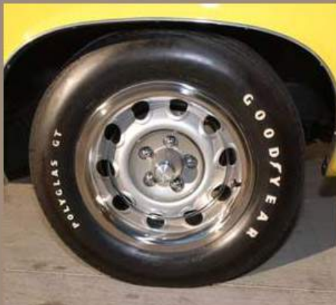
15" Rallye wheels were part of the Hemi'cudas option package, shod with E60-15 rubber.
