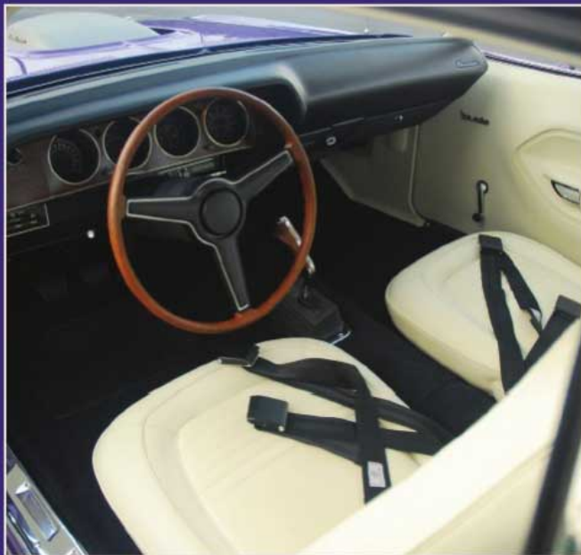
One of the most challenging areas of the restoration was this white interior, which made use of only original white plastic pieces.
