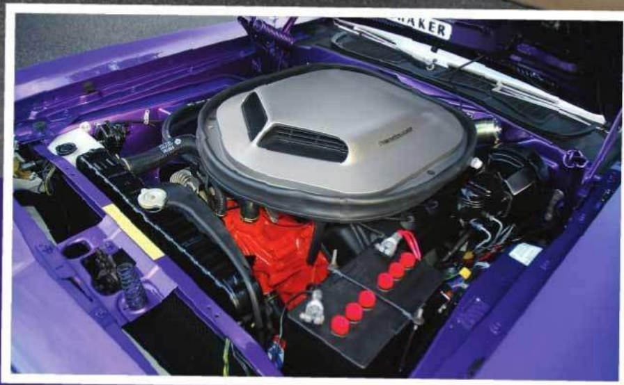
The 426 Hemi in 1970 had benefited from some changes, a big one being the swap to the hydraulic cam.
